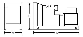
With 744RSL8054 LxWxH (mm): 5933 x 2212 x 2505 Dry Weight (kg) : 12590 Wet Weight (kg) : 13500 With 744RSL8058 LxWxH (mm): 5933 x 2212 x 2505 Dry Weight (kg) : 13090 Wet Weight (kg) : 14000
